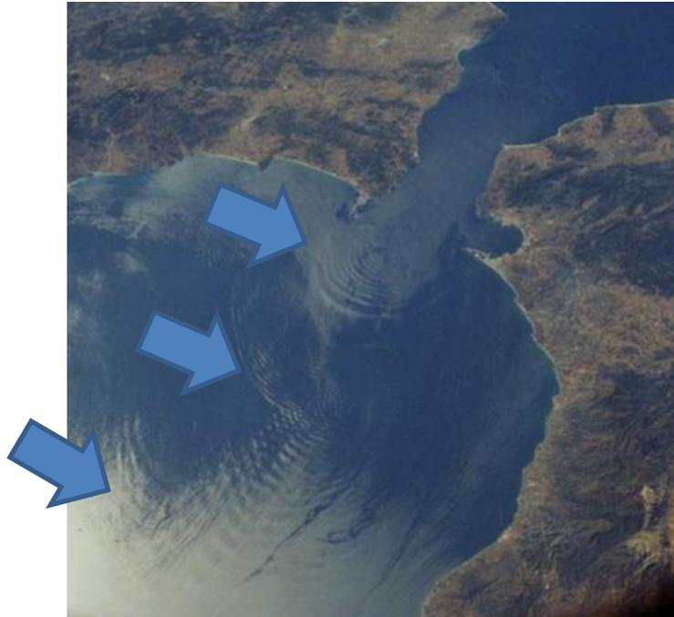
One of Paul's key aims of the space mission was to collect space imagery as evidence of internal ocean waves that did not appear to any large extent on the surface. Such "solitons" typically form on a surface separating two submerged water bodies of different density. The photographs showed the successive solitons at the entrance to the Straights of Gibraltar from two days before and one day before.
