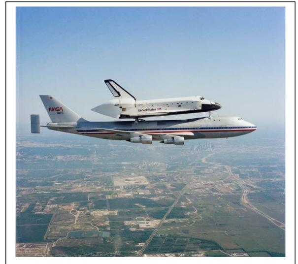
Without the Orbiter, the SCA needed to carry ballast to balance out its center of gravity. The SCA had an altitude ceiling of 15,000 feet and a maximum cruise speed of Mach 0.6 with the orbiter attached. A crew of 170 took a week to prepare the shuttle and SCA for flight.
